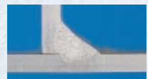
With start-up program – no fusion defects
