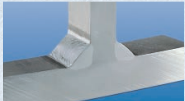
Base metal: AlMg 3 Sheet thickness: 25 mm Filler metal: AlSi 5, \varnothing 1.2 mm Shielding gas: Argon
